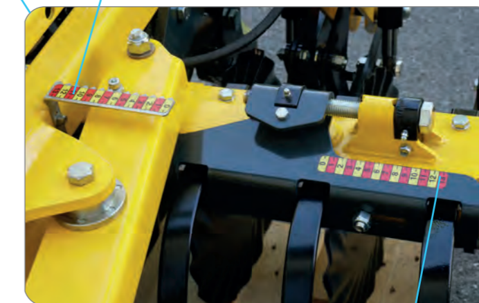
Spring adjustment on the horizontal plane
